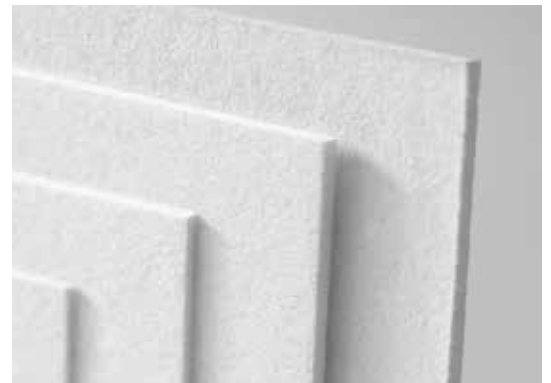
3 Layer: 210gsm cardstock(SBS) 2.5mm greyboard 300gsm Grey back cardstock(CCNB) Finish thickness is 2.9~3.1 mm
